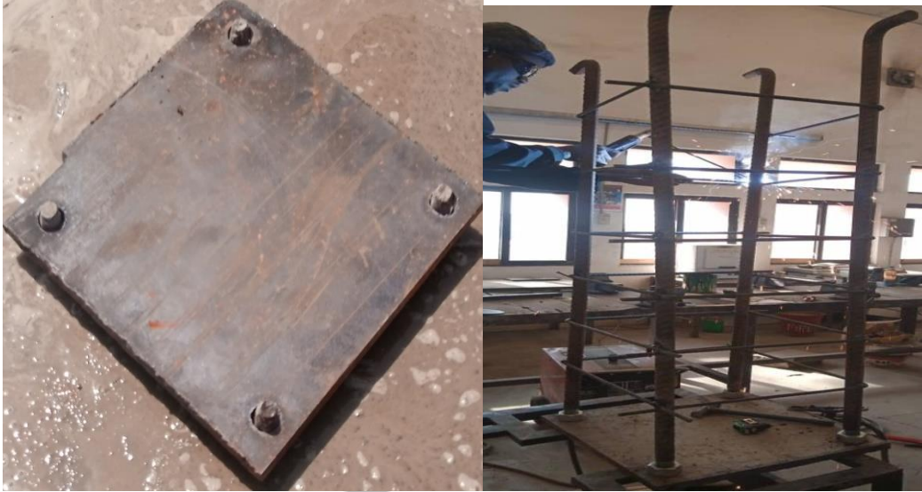
Plate 3.7 Base plate and foundation board
