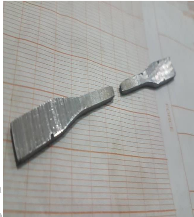
Plate 4.7 Galvanizes steel after tensile test
