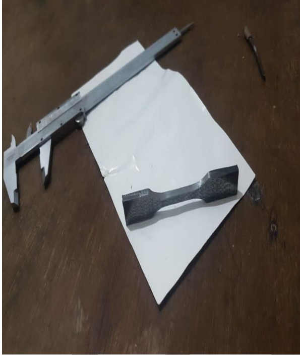
Plate 4.6 Galvanizes steel before the tensile test
